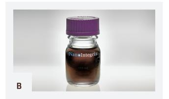
Figure 1. 5 mg of (A) MONO (B) and QUATTRO graphene in 100 mL of solution.
