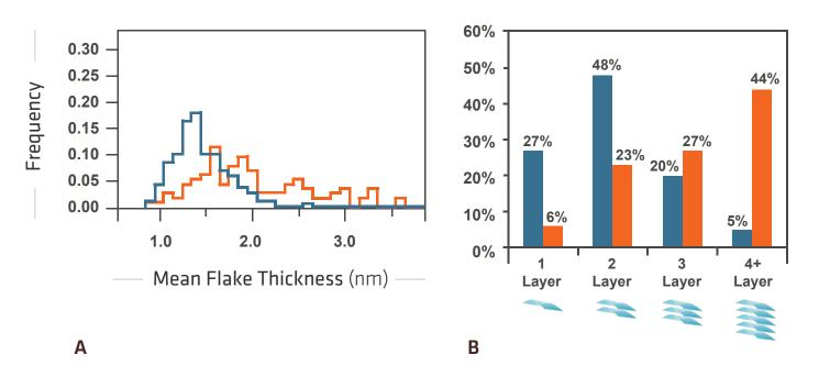
**Figure 2. (A)** Flake thickness histograms for MONO and QUATTRO products compiled by AFM analysis. The thickness of a single layer of graphene on an SiO<sub>2</sub> substrate, including adsorbed surfactant and water, is estimated to be approximately 1.1 nm<sup>\*</sup>. **(B)** Platelet-layer distribution of MONO and QUATTRO products. MONO Grade material consists of approximately 75% single and double-layer graphene. Approximately 71% of QUATTRO Grade material is triple layer or greater.
